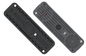
ND emitters eliminate drainage and refill effect, and improve efficiency in pulse irrigation. In order to achieve the ND function, the emitter opens at 0,40 bar and closes at 0,25 bar.
